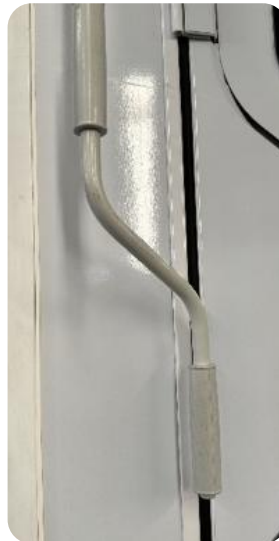
Use to rotate awning in and out
