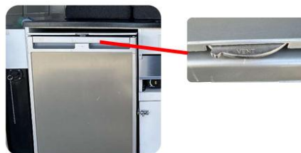
Fridge switch panel and vent dial
